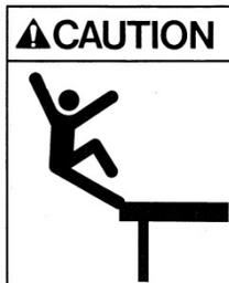
Circular collectors are usually exposed to the elements. The bridge and other access points may become slippery when wet or icy. Handrails and other safeguards must be in place when working on the equipment. Use care when access is necessary. **Do not work outside of the bridge handrails.** Wipe up grease and oil spills.
