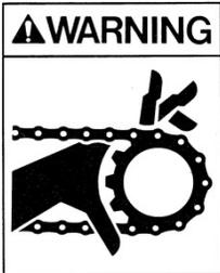
Guards cover several points on circular collectors to prevent personal injury from moving parts. If guards must be removed during maintenance procedures, use caution when operating equipment and replace guards when maintenance has been completed.
