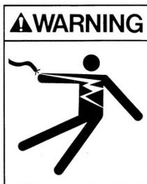
Electrical circuits may be energized in the torque overload control box even though the main power is off. Always check for live contacts before making adjustments within the box.
