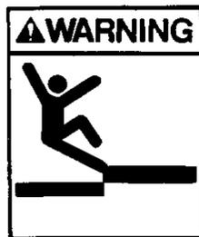
The access area for drive maintenance is below the bridge deck level. The difference in level will depend on the bridge design. A falling hazard exists. Use caution when in or near the access area.
