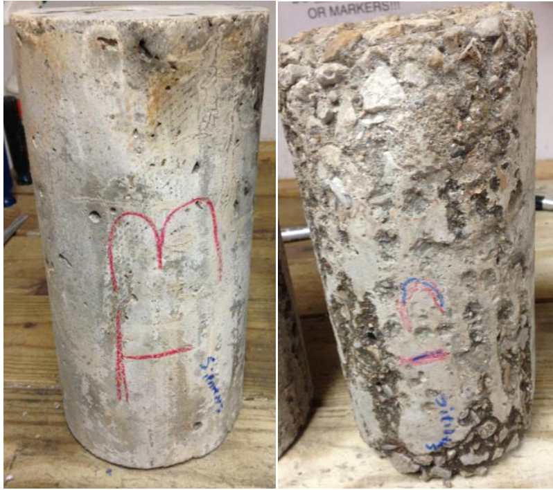
Figure 9 – Treated Sample (left) and untreated (right) after 24-months showing corrosion of concrete.
