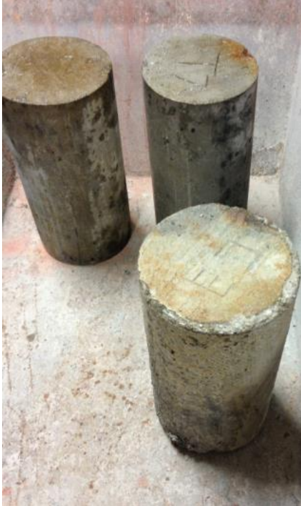
Figure 7 – Treated Samples (back) showing 0.3% mass loss after 12-months compared to untreated Sample (front) showing 2.6% mass loss.
