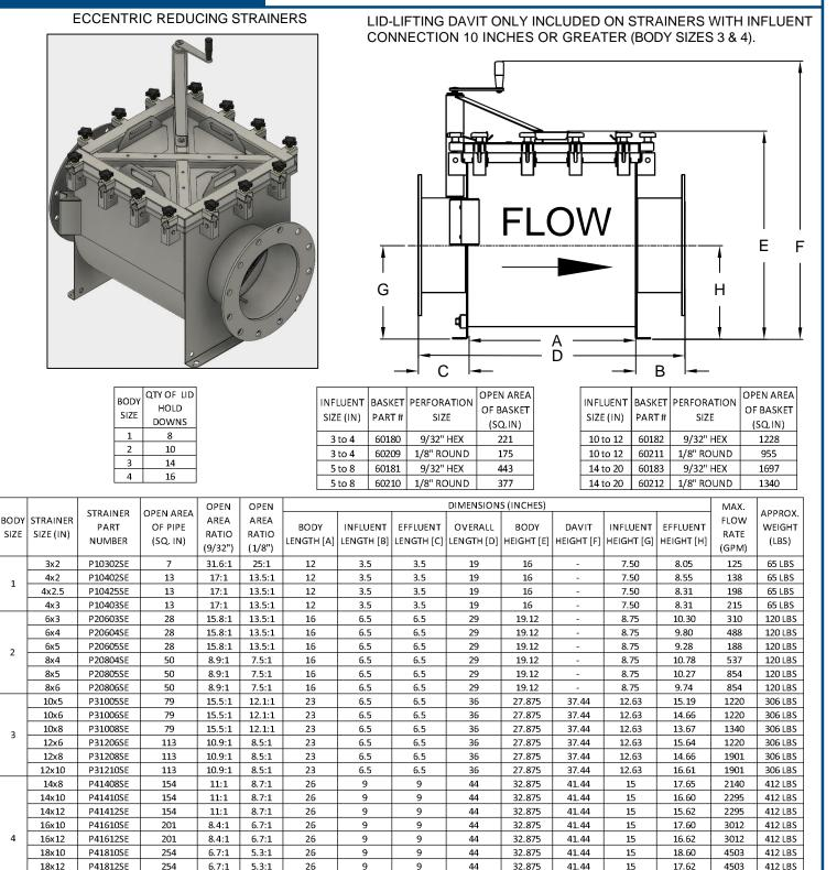
STRAINER BODY SHALL BE CONSTRUCTED OF T316 MATERIAL NOT LESS THAN 1/8" IN THICKNESS. FLANGED CONNECTIONS ARE CONSTRUCTED OF T316 STAINLESS STEEL PIPE & WELDED FLANGES. FLANGED CONNECTIONS SHALL BE ANSI STANDARD DIMENSIONS. OTHER STRAINER SIZES AVAILABLE UPON REQUEST.
