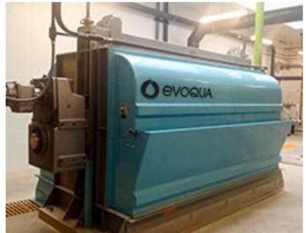
Evoqua can supply shaft-mounted drives providing greater access to machinery than traditional drive chain applications. Our removable rear splash housing section allows clear access to the baskets and carrier chains.
