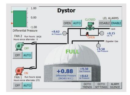
The operator interface is a user-friendly tool that allows system status to be immediately determined at a glance. The PLC can interact with the existing SCADA systems and is capable of interacting with other digestion equipment, including co-generation systems.
