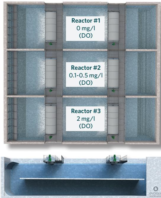
Typical VLR system Plan View and Cross-Section View utilizing surface mounted disc aerators providing both aeration and mixing.
