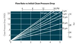
Water Flow Rate/10" cartridge (GPM)
