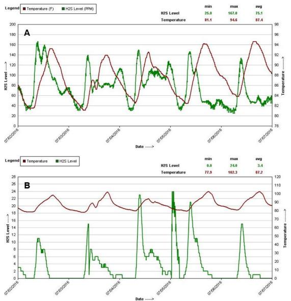
Figure 1 – Untreated Atmospheric H<sub>2</sub>S. A) Scrubber Inlet, B) Scrubber Outlet.
