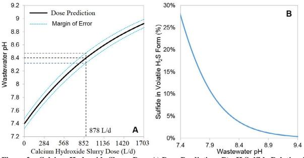
Figure 2 – Calcium Hydroxide Slurry Dose A) Dose Predictions B) pH Sulfide Relationship
