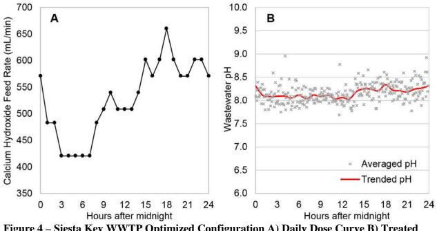
Figure 4 – Siesta Key WWTP Optimized Configuration A) Daily Dose Curve B) Treated Wastewater pH
