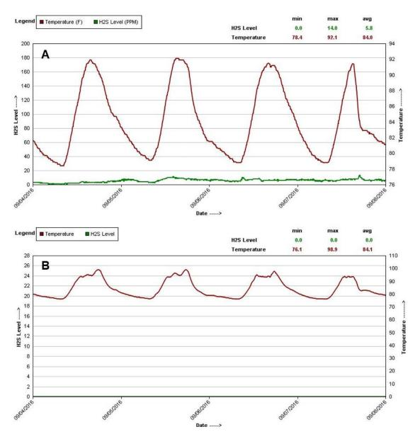
Figure 5 – Treated Atmospheric H<sub>2</sub>S. A) Scrubber Inlet, B) Scrubber Outlet
