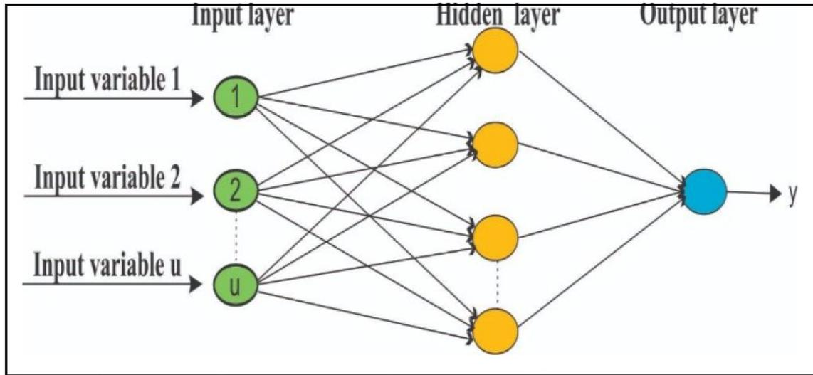
**Figure 1: Layer structure of an ANN model**
